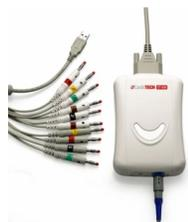
PC Based EKG machines generally plug in to a PC via a USB connection or wireless via Bluetooth. You can easily print to plain paper or simply save the test results on the PC as a PDF. These machines tend to carry less cost but must use a PC to operate. Make sure you ask if the EKG you select is compatible with the latest version of windows.
