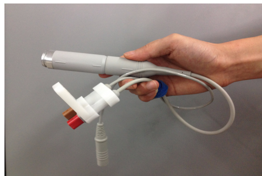
FIGURE 11-11 Connecting the Transducer Cable and Camino Adapter
