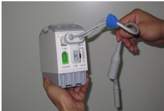
FIGURE 11-13 IBP Cable Inserted into VPS
