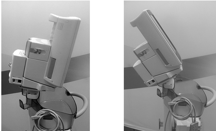
FIGURE 4-39 Pivot - Monitor pivots 360° around, forward, and backward
