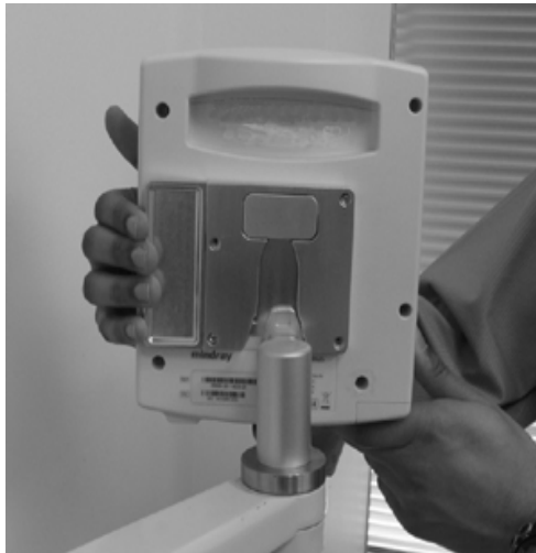
FIGURE 4-28 V Hub on a Wall Mount Post
