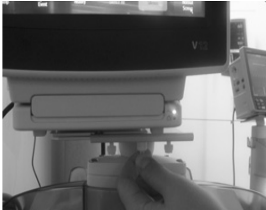
FIGURE 4-22 Removal from Rolling Stand
