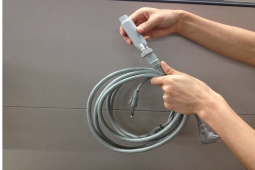
FIGURE 11-12 Connecting the Bedside Monitor Connector and Camino Adapter
