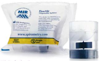
The disposable turbine is fully compliant to ATS/ERS accuracy standards, and unlike most other transducers it is not affected by ambient temperature, humidity and pressure
