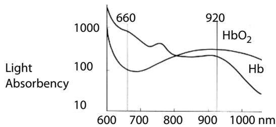
Here, an infrared beam at a wavelength of 920 nm and a red beam at a wavelength of 660 nm are alternately flashed ON and OFF and transmitted through the measurement section (in this case, a finger). The light-volume ratio of these transmitted lights is calculated to enable measurement of the level of oxygen saturation.
