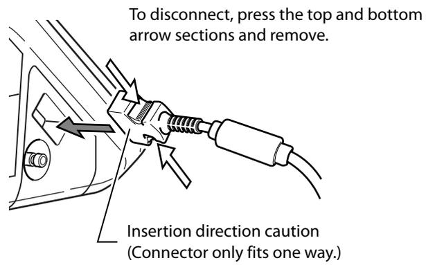
2. Insert the SpO<sub>2</sub> sensor onto the extension cable, lower the cover, and lock it.
