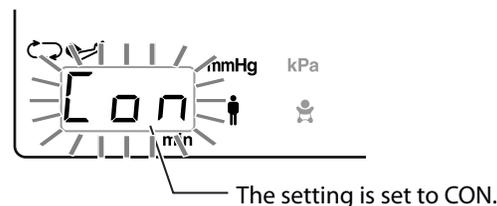
3. If you do not press a switch for 10 seconds or press **Cuff Start/Stop**, **Alarm Silence** or **Cuff Interval**, **Setting Mode** ends and the display returns to the basic screen. (Settings are not finalized until you press the **Cuff Start/Stop** switch.)
