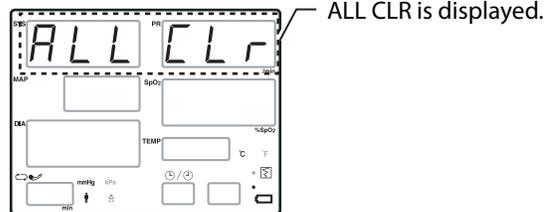
Hold down the **Alarm Silence** switch for at least 3 seconds.
