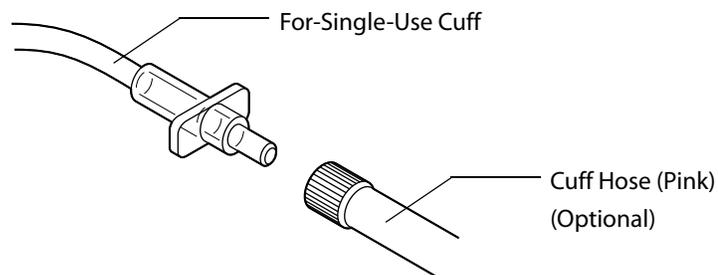
**Note:** Make sure that the connectors are tightly connected, as air leaks will prevent accurate measurement.
