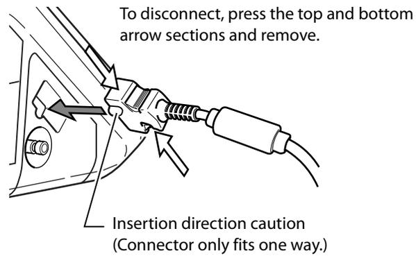
2. Insert the OXISENSOR® onto the extension cable, lower the cover, and lock it.
