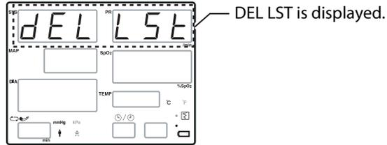
Hold down the **Alarm Silence** switch for at least 3 seconds.
