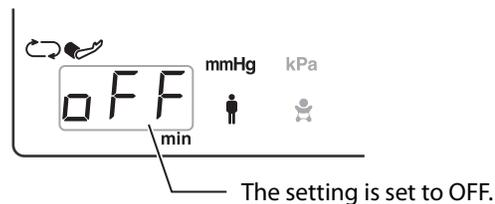
3. If you press the **Cuff Interval** switch or wait for 10 seconds without pressing any other switch, **Setting Mode** ends and the display returns to the basic screen.
