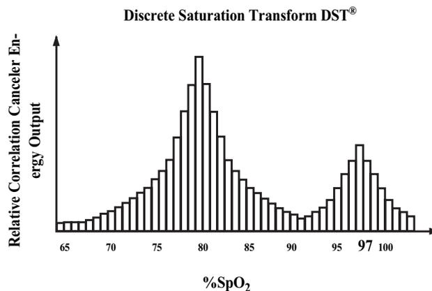
The DST plot has two peaks: the peak corresponding to the higher saturation is selected as the  $SpO_2$  value. This entire sequence is repeated once every two seconds on the most recent four seconds of raw data. The MS board  $SpO_2$  therefore corresponds to a running average of arterial hemoglobin saturation that is updated every two seconds.
