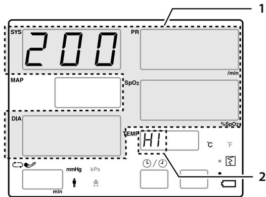
**Figure 8-1: Example of the SYS upper limit Display**
