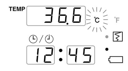
Body temperature measurement has two built-in measurement methods, estimated and actual measurement. Measurement always starts with the estimated measurement, but under the conditions below, measurement automatically switches to actual measurement. From that point in time, the body temperature unit display flashes. Observe the display until the value stops changing (3-5 minutes), indicating the final temperature.
