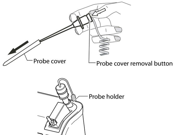
Return the body temperature probe to the probe holder on the top of the main unit.
