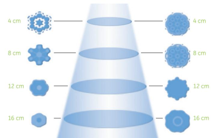
At greater depths, a conventional 7-crystal transducer has a narrower focal region.
