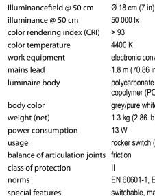
50 000 lx > 93 4400 K electronic converter 1.8 m (70.86 in), US hospital graded plug polycarbonate & acrylonitrile butadiene styrene copolymer (PC & ABS) grey/pure white 1.3 kg (2.86 lb) 13 W rocker switch (I/0) at the arm Ш EN 60601-1, EN 60601-2-41 switchable, maintenance free, US hospital graded plug fastening pin (Ø 16mm) wall mount
